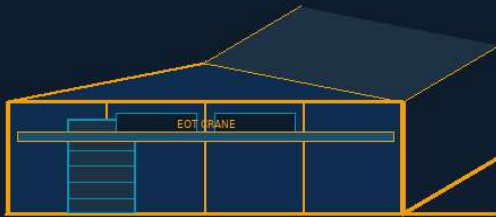
IB-3 Warehouse (30m span)
